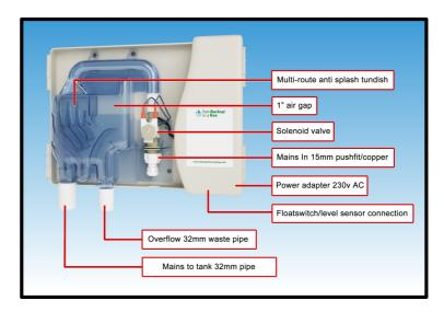
For this reason all mains backup devices must have an air gap where the mains water flows into the rainwater tank. The air gap in this system is an anti-splash tundish and overflow incorporated into one; the transparent blue moulded part. The level sensor is provided with 15 metres of cable and uses a push connection under the right hand panel.
